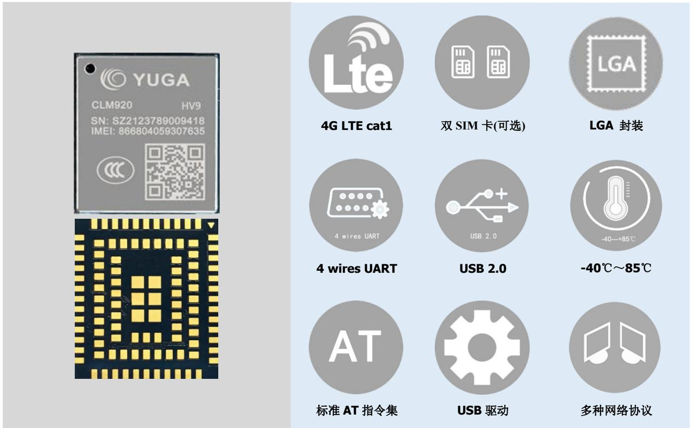
The image displays the CLM920\_HV9 module and its key features. The module is shown in two views: a top view with the YUGA logo, model number, SN, and IMEI, and a bottom view showing the LGA package. The features are listed in a grid of icons:
