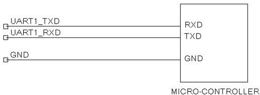
Figure 5-1 UART interface and microprocessor connection reference design
